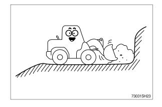
Avoid parking and stopping on a slope. Lower the bucket to the ground and block the tire when parking.
