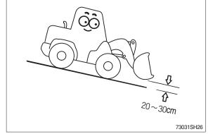
Steering of the machine while traveling on a slope is dangerous.
